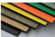
**HPL board (High Pressure Laminate)** is considered to be one of the most durable decorative surface materials. It is manufactured by simultaneous pressing of layers of cellulose fiber material impregnated with thermosetting resins and specially pre-treated craft paper subjected to both pressure and heat. The resulting laminate is strong, durable and water resistant.
