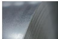
**Electric galvanization** aims at covering the surface of steel products with a zinc coating in order to protect them against corrosion. In urban environmental conditions a zinced coating shows better resistance to steel corrosion than the one which hasn't been zinced. The final effect is getting a smooth steel surface of golden or silver color. Properly made zinc layer can endure from 2 to 10 years depending on its thickness, aggressiveness of the environment and mechanical erosion.
