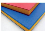
**HDPE sheet** is extremely strong against bad weather conditions and mechanical damage. The material's durability makes it a perfect match for a variety of applications. It is widely used on commercial playgrounds.
