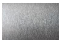
**Stainless steel** also known as inox steel or inox is a steel alloy with a minimum of 10.5% chromium content by mass. It is notable for its corrosion resistance. Stainless steel is a protection system itself, it does not require other surface coatings.
